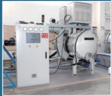
真空炉 Vacuum Furnace
